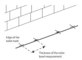
5. If using the 'L' shaped bracket assembly, place the front edge of the bracket on the inside mark, then mark the screw hole position to secure the bracket to the floor. Repeat on the other side.
