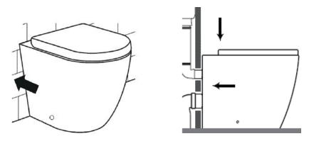
9. Once aligned, secure the toilet pan into position using the fixings provided, do not overtighten. Finish by pushing on the screw covers.
