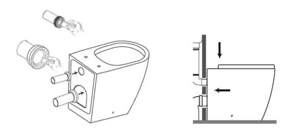
3. Ensure that the toilet pan is level and backed fully against the wall / WC unit, then mark on the outer edge of the pan (at both sides), align with each fixing hole located in the side wall of the toilet pan.
